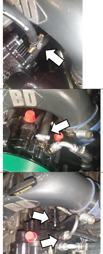
Acquire supplied fan shroud bracket, and shroud spacer, and assemble as shown above right.
