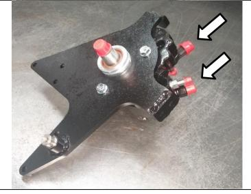
Mount pump and bracket to engine, using one (1) M8x25mm bolt and four (4) supplied M8x50mm bolts with four (4) flange nuts.
