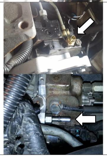
**5.9L Trucks:** Install supplied -8JIC swept fitting (PN 1502038) into the low-pressure fuel feed line using supplied gear clamp.
