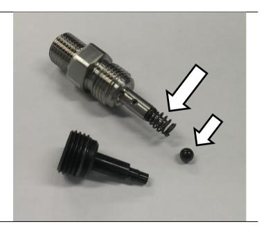
Reinstall ball bearing and supplied fitting assembly into port where plug was removed.
