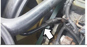
Using the T50 Torx bit, remove plug from lower driver's side rear of original cp3 pump in the truck.
