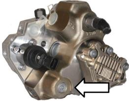
Transfer spring from plug to the supplied high-pressure fitting (PN 1500680) as shown.
