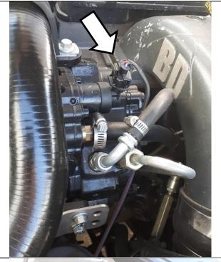
Mount controller in a safe area in the engine bay away from heat sources or belts and pulleys.
