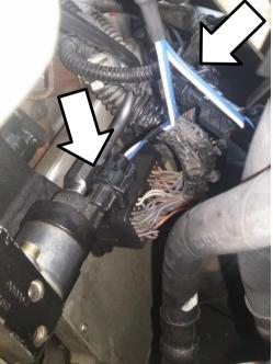
Route the supplied harness up to the second CP3 pump and plug it into the pumps metering unit.
