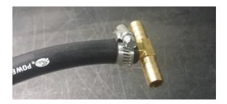
**Note** If using a fuel distribution block, connect the fuel hose to the supply port of the block instead of splicing into feed hose.
